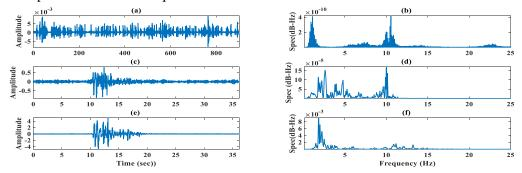
Fig. 2. Acceleration and spectrums, (a,b) bridge, (c,d) frame-intact, and (e,f) frame-damaged
