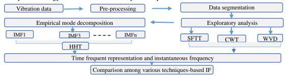
Fig. 1. Overall diagram of the work methodology
